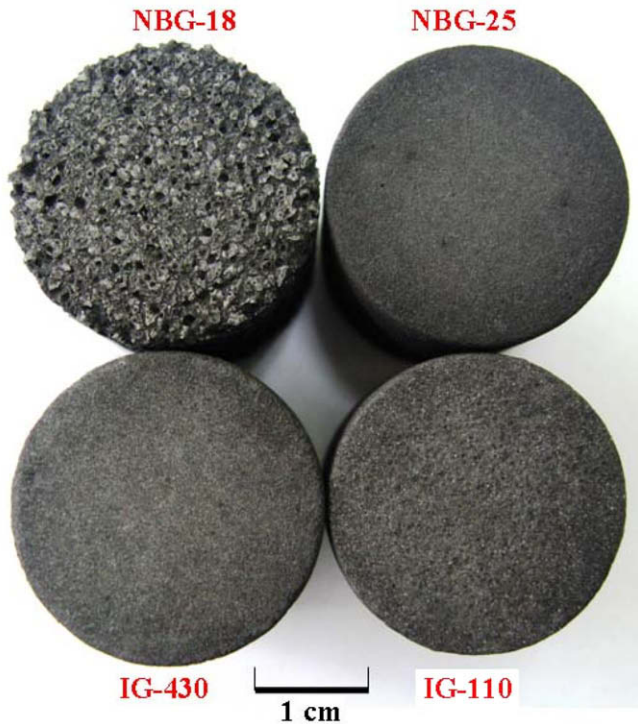
Fig. 6. The optical photos of the graphite specimens oxidized at 808 °C in dry air at a flow rate of 10 l/min (weight loss: 10%).
